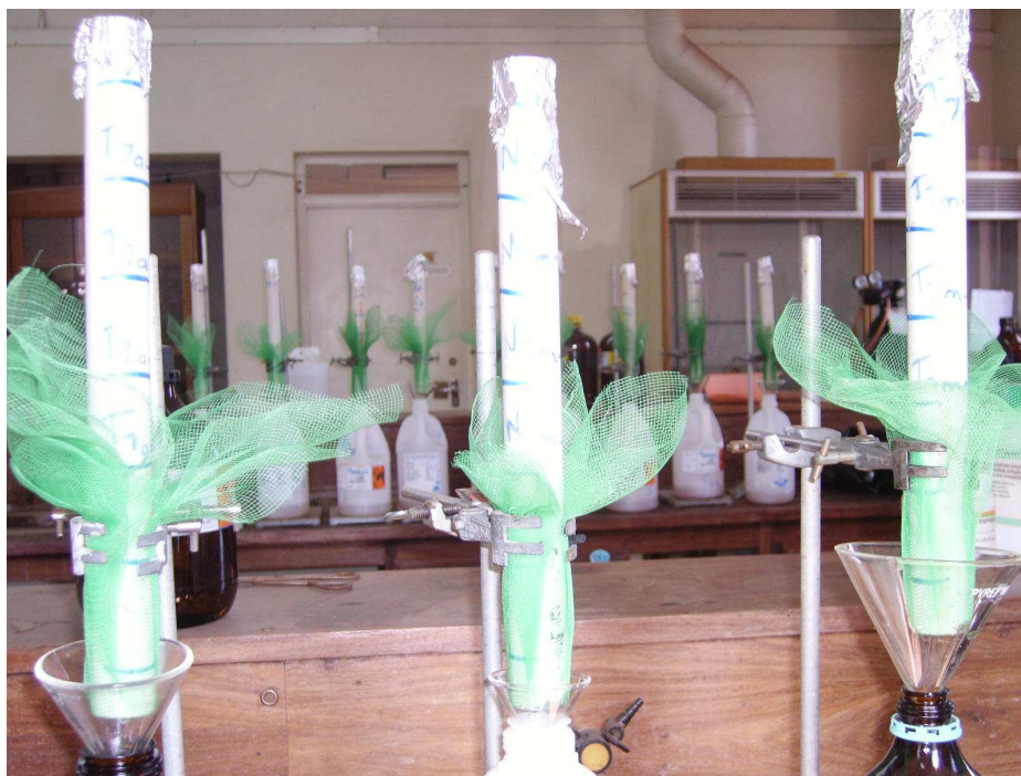
Figure 18: Hand-packed soil columns for leaching experiment
